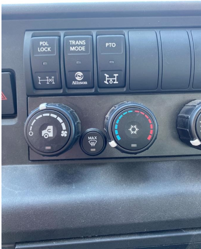
PTO switch on dash at center
