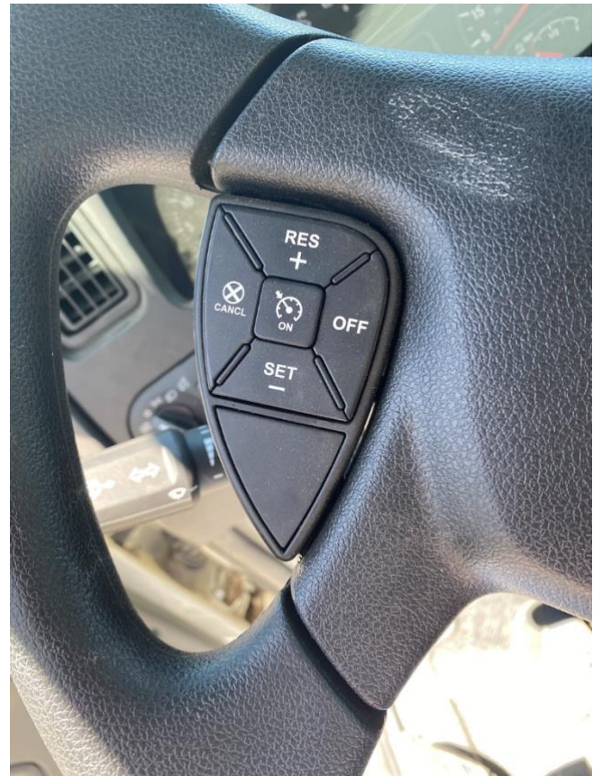
Steering wheel cruise control switches, on (center), up (Res + at top), and down (Set – at bottom)
