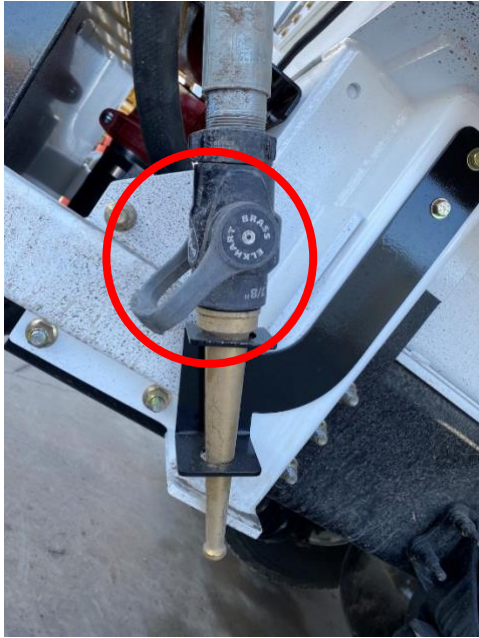
Swivel shutoff valve at nozzle head.
