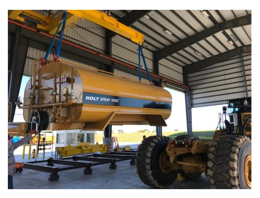
Tank should be rigged with a slight tilt towards back of tank.
