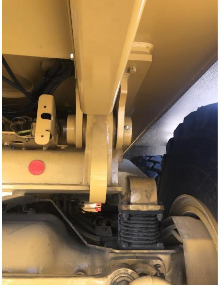
Lower tank into place and install pivot pins.
