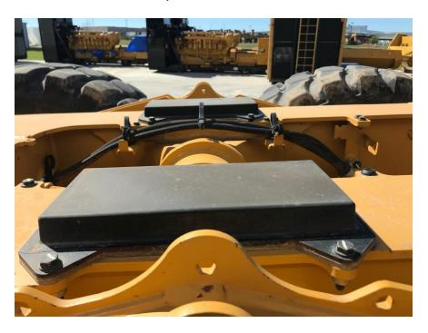
Tube style frames will need to have mount tabs welded in place to mount pad after tank is installed.
