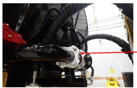
When lowering the tank onto truck, water pump outlet coupling will need to be removed on Cat 740 and Cat 745 models for hydraulic lines. Use of tag lines is part of a safe lift.
