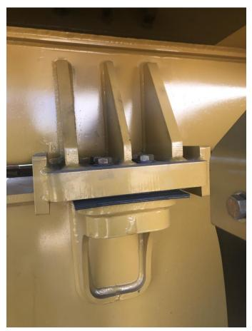
Install rubber isolator between chassis and tank mount, then bolt front mounts in place.
