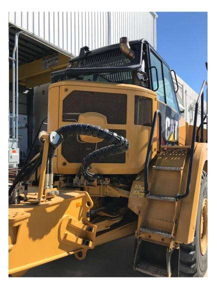
Cab harness and return line to tank will route through main loom wrap that houses truck to rear chassis connection.
