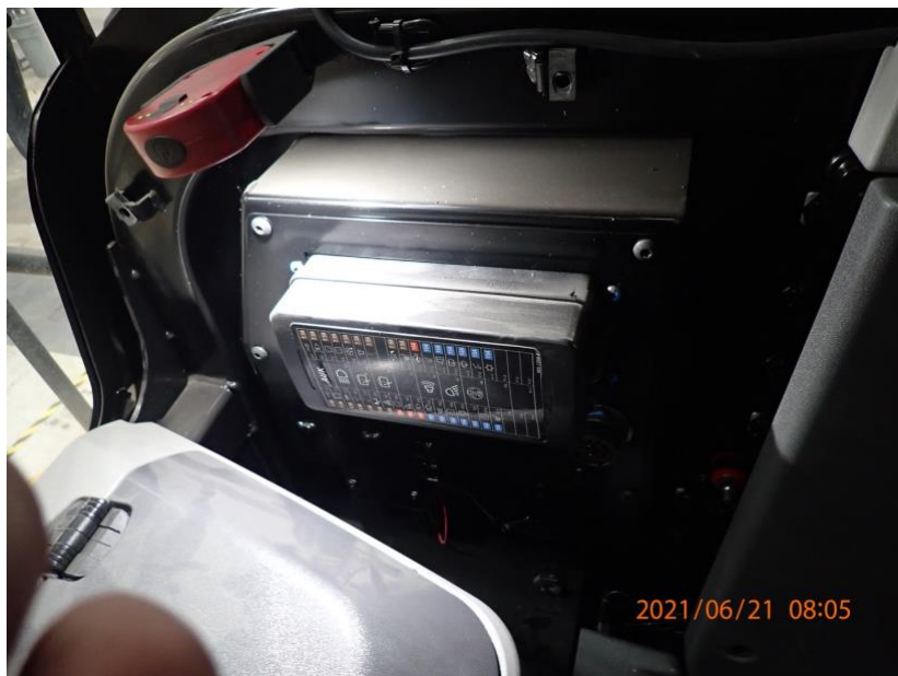
Remove panel cover around fuse box
