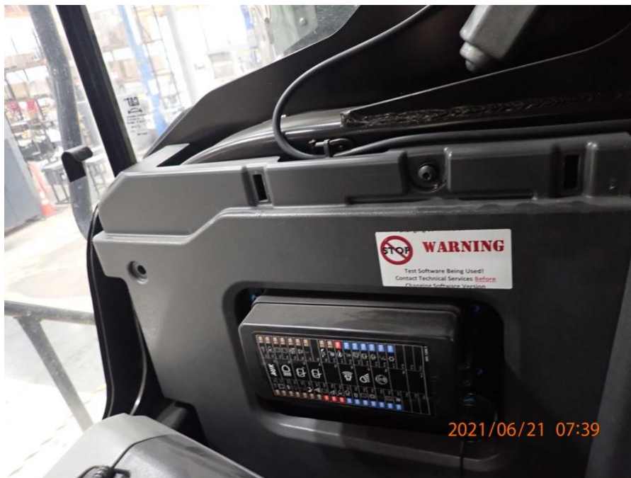
Remove top dash panel over fuse box (behind right side driver's seat)
