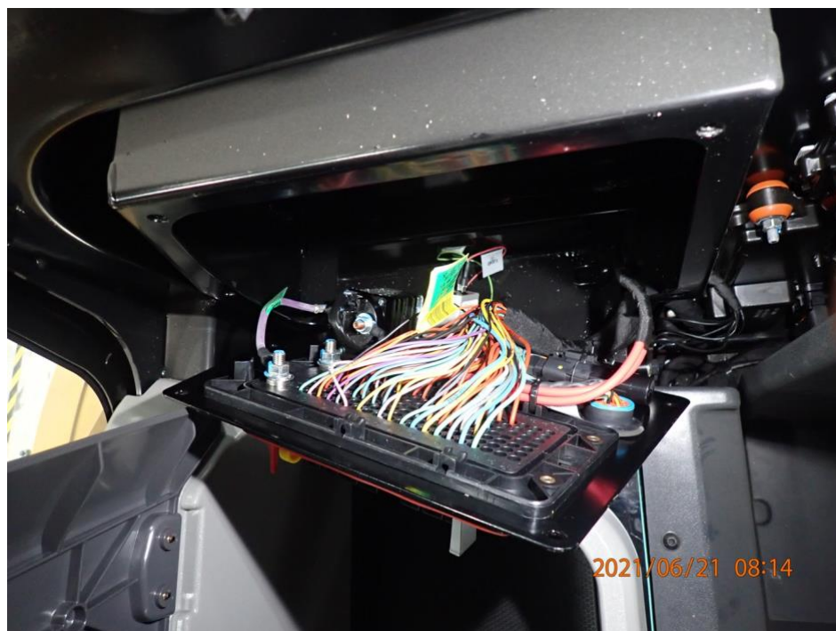
Remove fuse panel box
